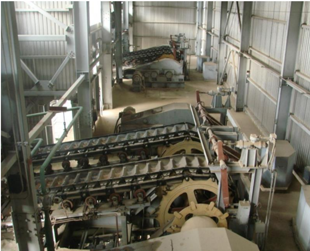
12: Blast furnace's pig iron casting machines no. 1&2 (99% completed)
