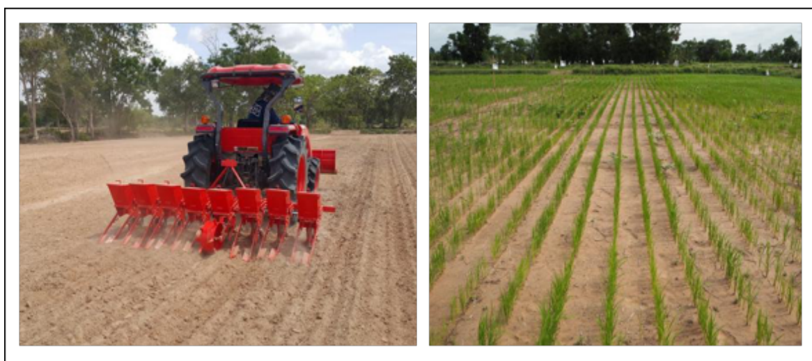
Photo 6. 1 Left: rice seed dibbling machine; right: rice field planted using the dibbling machine.
