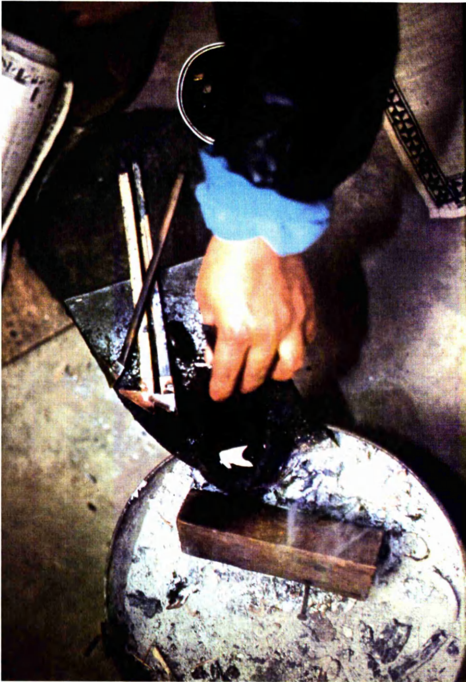
Photograph 5: The tools of batik production. Each woman possesses a selection of batik tools; this woman has a specially designed tool rest made by her husband from an old piece of metal, and attached to her bucket of hot ashes.
